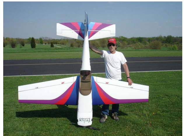
Our buddy Mr. Lee Buck sporting his 33% Hanger 9 Extra 330L, Brison 6.4 Twin(104cc) Gas Engine, 97" Wingspan, Hitec Digital Servos, Duralite Powerbox and Batteries
