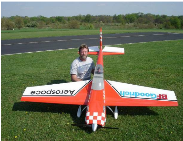
Gary McLeod posing his AeroWorks Extra 330L in Patty Wagstaff Colors, DA-100 Gas Engine, 29 lbs., 104" Wingspan, Hitec Digital Servos
